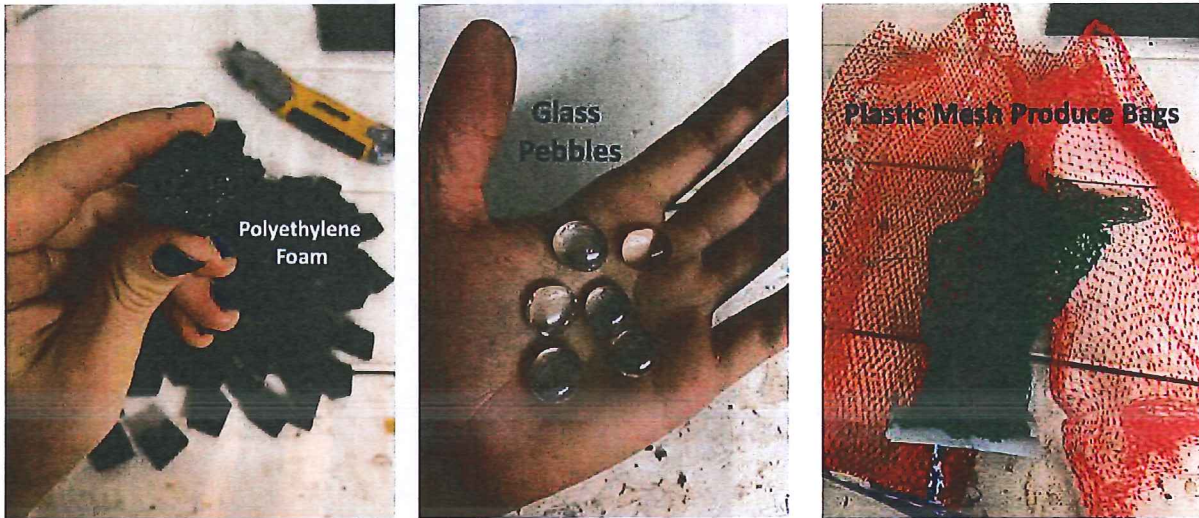
Figure 7. Digester Floater Components. November 23, 2019.
